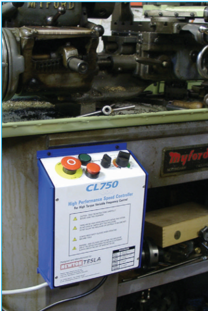
1. Newton Tesla Variable Speed Inverter drive fitted to Myford Super seven
