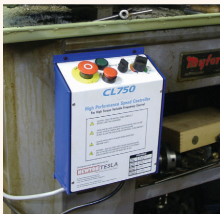
A Newton Tesla VFD package fitted to a Myford Super 7 lathe.
